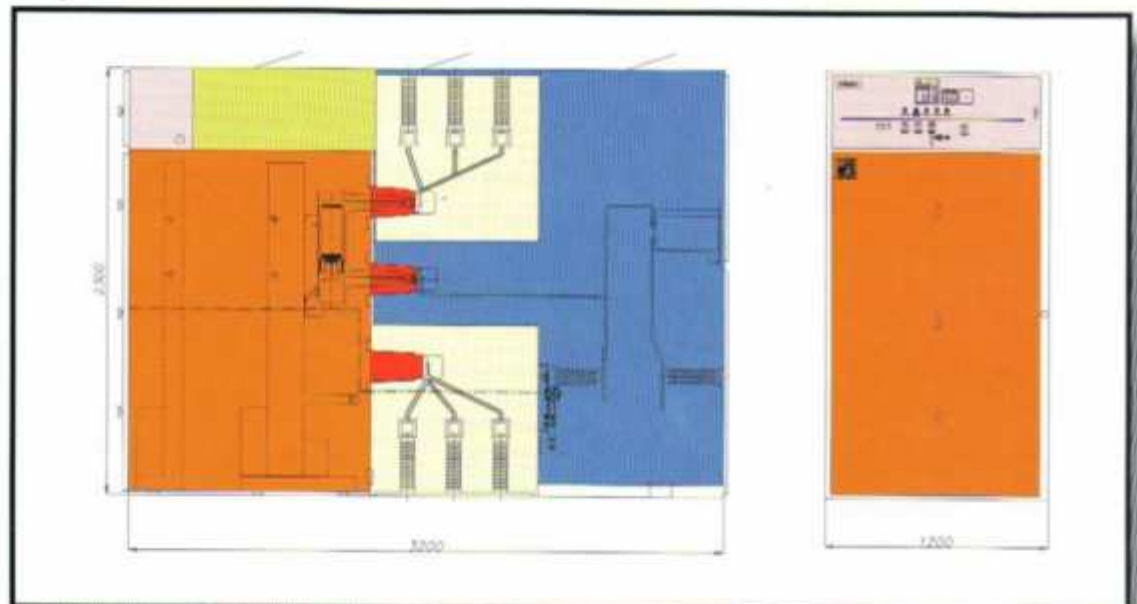
PVP - 702 36kV DOUBLE BUSBAR OUTGOING PANEL
